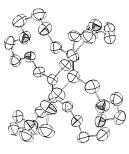
a rigid group. For 1091 observed structure amplitudes measured with MoK $\alpha$  radiation using  $\odot$ -2 $\odot$  scans to 40.0 deg, the final residuals were R=0.056 and wR=0.070.
