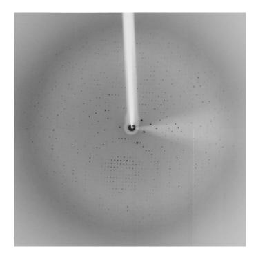
**Figure 2** X-ray diffraction image from a native *P. horikoshii* LeuRS-tRNA<sup>Leu</sup> crystal. The edge of the detector corresponds to a resolution of 3.2 Å.
