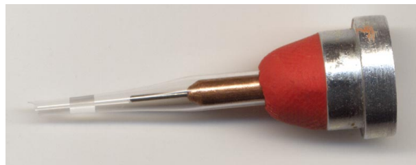
Figure 4 Loop-mounted crystal enclosed in capillary.
