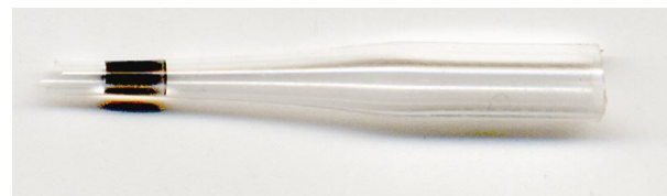
Figure 2 Cut 1.5 mm capillary (with solution added).
