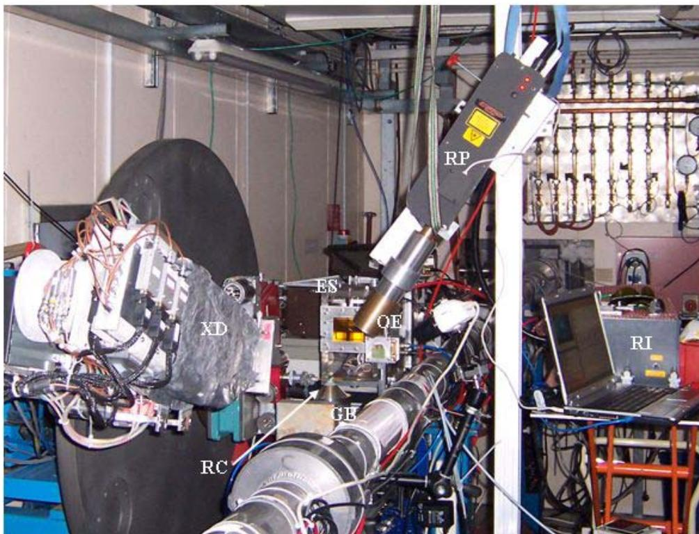
**Figure S1:** Picture of the Raman-XRPD experimental setup in the operating mode. XD: X-ray detector; RI: Raman instrument; RP: Raman probe; OE: optical expander; RC rotating capillary; GB gas blower; ES: empty space
