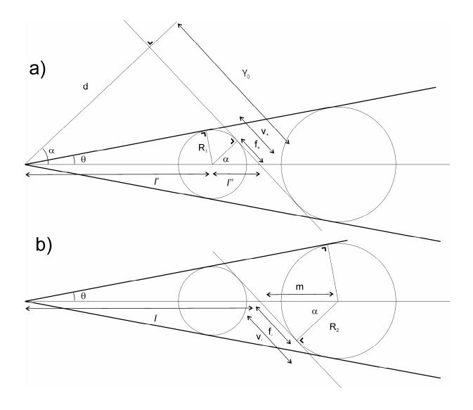
Figure 1. Two Dandelin spheres relevant to the case of ellipses, and definition of some symbols.
