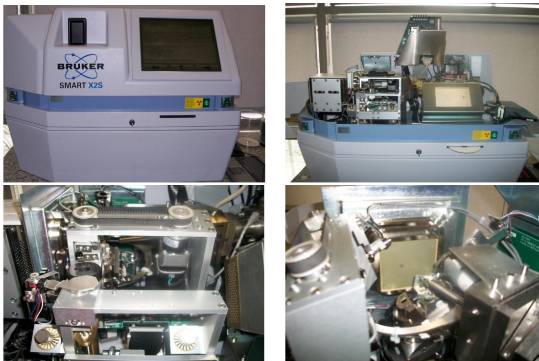
Figure 1: The Benchtop Bruker SMART X2S: external view (top left), cover removed (top right), patented sample loader (bottom left) and detector with beam stop (bottom right).
