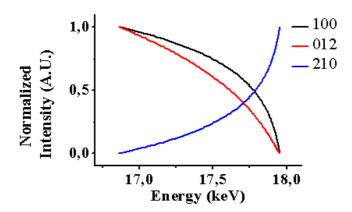
Three structure factors as a function of Energy. When comparing with Figure 3 in the paper, one notices the importance of using 'scan number' as a variable for the demodulation technique.
