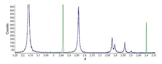
Black curve is the  $ZrO_2$  sample measured in a 0.3 mm capillary on the HRPD instrument at 0.50114Å. Blue curve is the same capillary measured on the 2 dimensional Pilatus detector with a wavelength of 0.73536Å. For clarity the ultimate resolution of the HRPD diffractometer is shown with an LaB6 lineshape standard at 0.50114Å (Green curve).
