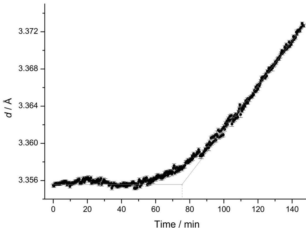
**Figure S1.**  $d$ -spacing of the '002<sub>2H</sub>' diffraction peak as a function of discharging time.
