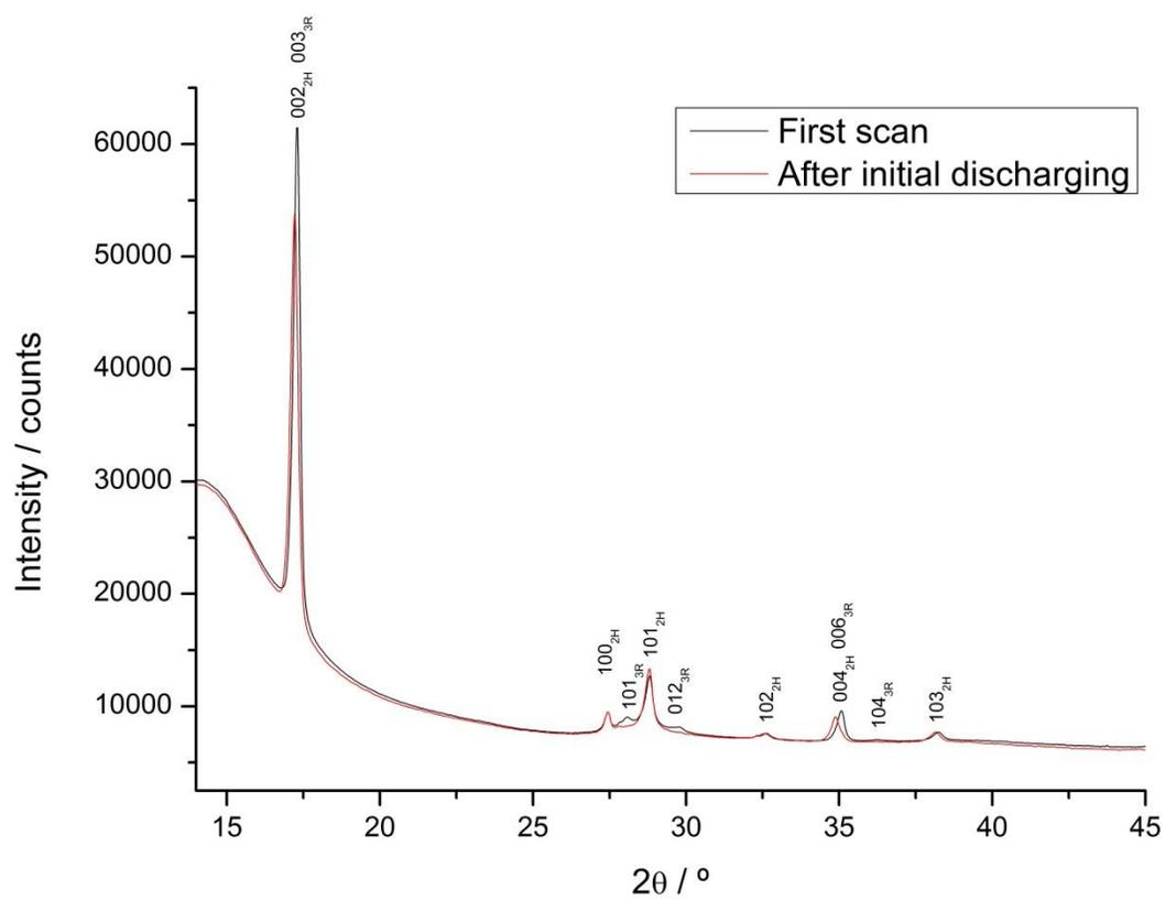
**Figure S2.** XRPD patterns of the graphite electrode in a lithium-graphite micro-battery cell.
