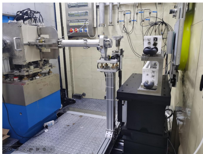
Figure 7 The sample stages and sample changer in the sample hutch of the VSANS instrument.
