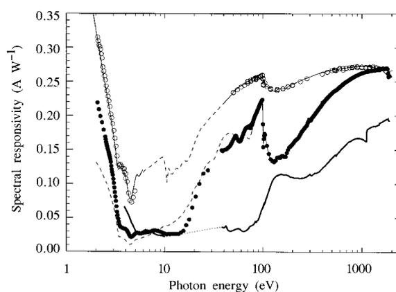
**Figure 1** Spectral responsivity of a silicon n-on-p diode (AXUV100G; open circles) and PtSi/Si (closed circles) and GaAsP/Au (G2119; thick solid line) Schottky barrier diodes measured against SYRES. The thin lines represent a model calculation for the silicon diodes; dashes indicate the spectral regions where the model is not reliable due to a lack of optical data.
