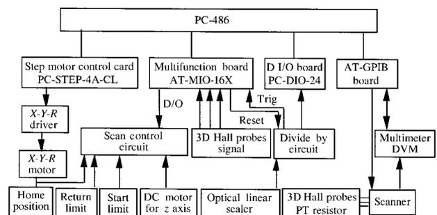
**Figure 1** The hardware architecture of the three-orthogonal-Hall-probe system with the 'on the fly' mapping method.
