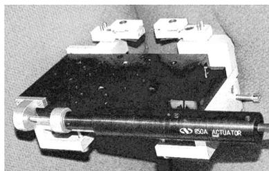
**Figure 1** Photograph of the tensometer. The Newport 50 mm travel linear slide is driven by a Newport 850A actuator. At the top of the photograph the jaws of the tensile stage can be seen. These conform to ASTM Standard D3379.
