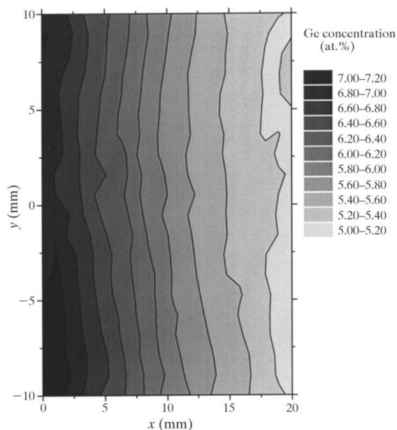
**Figure 8** Concentration profile of Ge in Si calculated from the diffraction measurements for the SiGe graded crystal (Institute of Crystal Growth, Berlin, sample 39.27).
