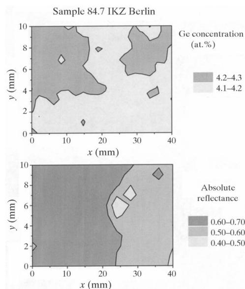
**Figure 9** Concentration profile of Ge in Si calculated from the diffraction measurements for the doped crystal (Institute of Crystal Growth, Berlin, sample 84.7).
