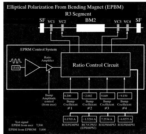
Figure 4 Display of the present phase EPBM graphic user interface.
