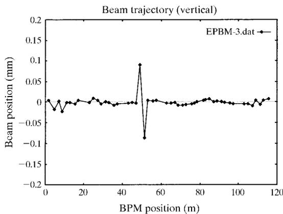
Figure 2 A typical local bump was generated in the third-section storage ring under regular user shift lattice.
