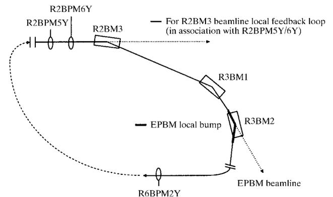
Figure 5 Schematic layout of the test run of the EPBM with local feedback loop.
