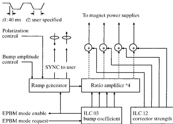
Figure 3 Functional block diagram of the EPBM control electronics.
