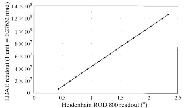
**Figure 4** A plot of the test results correlating the performance of the LDAE with a Heidenhain ROD-800 optical encoder.
