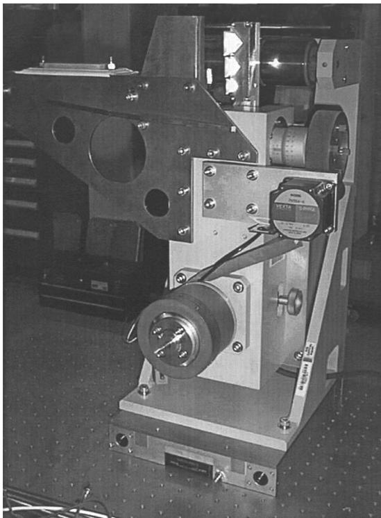
**Figure 3** A photograph of the monochromator together with the mounted LDAE.
