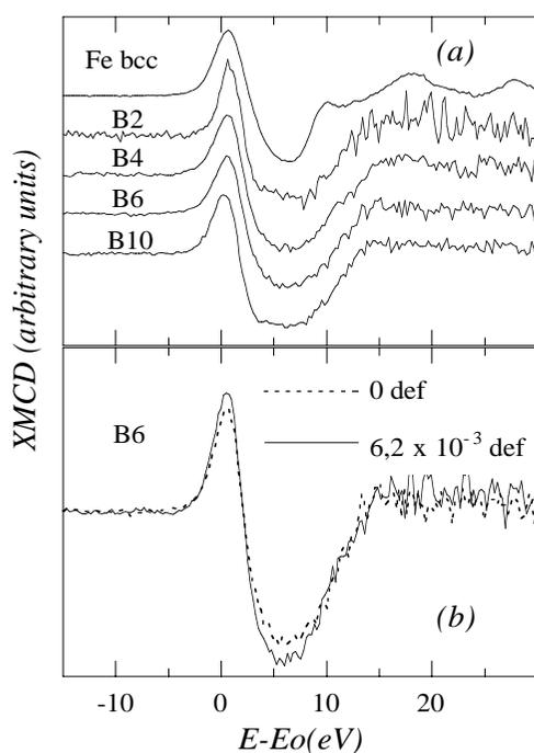
**Figure 1** (a) X-ray Magnetic Circular Dichroism spectra normalized to the peak to peak amplitude recorded without stress of B2, B4, B6 and B10. The spectrum of Fe bcc is shown for comparison. (b) X-ray Magnetic Circular Dichroism spectra for B6 sample with and without stress
