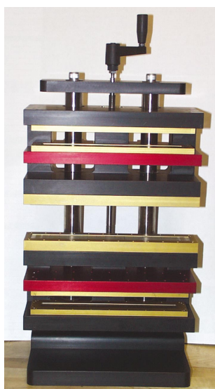
Figure 5 A prototype counterforce system. The black jaws hold the main magnets (gold keepers in center) and the moving counterforce magnets (gold keepers at bottom and top). The red fixtures hold the stationary counterforce magnets. The lead screw is 12.7 mm in diameter with a pitch of 0.787\text{ mm}^{-1} . The crank handle is 65 mm from axis to handle axis.
