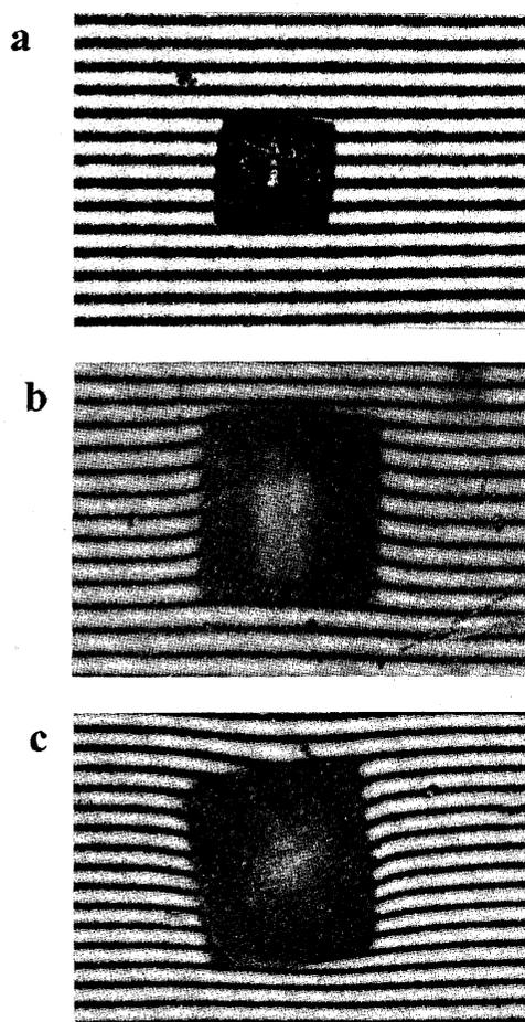
**Figure 4** Interferograms around the tetragonal crystal of lysozyme. Conditions: 40.2 mg lysozyme/ml in 50 mM sodium acetate buffer (pH4.5) at 20°C. (a) Equilibrium (0.36 M NaCl); (b) growth (0.40 M NaCl); (c) dissolution (0.30 M NaCl).
