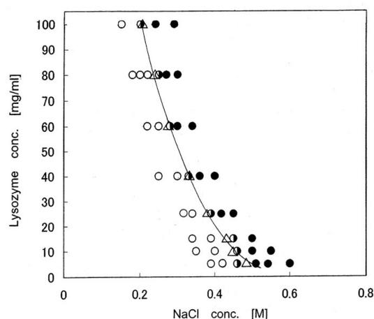
**Figure 5** Solubility curve of tetragonal lysozyme crystal as a function of NaCl concentration at 20°C. Circles represent the conditions where a tetragonal lysozyme crystal apparently dissolved (open circles) and grew (solid circles). Open triangles represent the equilibrium conditions determined by bracketing the fringe shift values nearest 0 at the dissolution and the growth.
