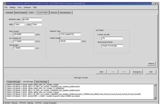
Figure 6 Current Status tab. Status of the storage ring, the beam shutters, X-ray intensity etc. are displayed.
