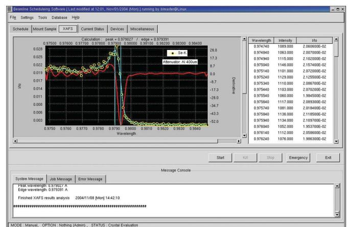
Figure 5 XAFS tab. A graphical plot of XAFS measurements is displayed. The results of profile analysis, i.e. peak, edge (maximum, minimum derivative) wavelengths and derivative plot are superimposed.
