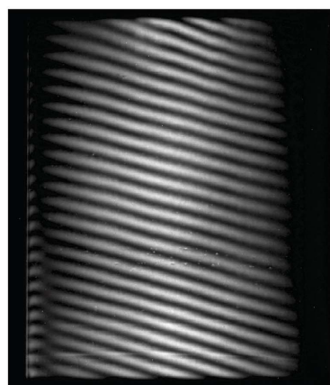
Figure 1 (a) Two-crystal X-ray interferometer and (b) a 25\text{ mm} \times 30\text{ mm} interference pattern obtained with 35 keV X-rays. The fringe visibility was 50%, which is good enough to obtain phase-contrast images.
