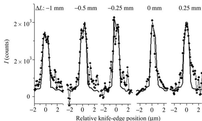
**Figure 2** Beam intensity profiles as obtained by derivation of knife-edge scans for five different values of the mirror–knife-edge distance  $L_{KE}$  (closed points). The variation  $\Delta L_{KE}$  with respect to a reference value coincident with the focal distance  $L_F$  is marked on the different profiles. For each profile the abscissa indicates the knife-edge translation. The full line represents calculations (see text).
