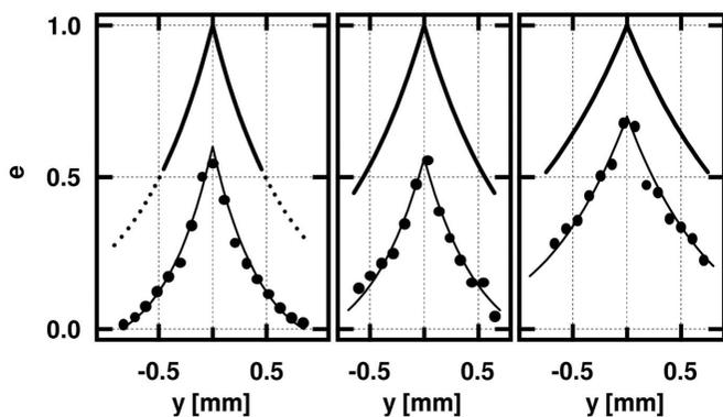
**Figure 8** Refraction efficiency  $e$  for the focusing of X-rays depending on the off-axis position  $y$  in lenses (from left to right) 35/1/SU8, 35/1/pmma and 35/2/pmma. The dots are the measured points, the thin line is the simulation by use of (47) and the thick lines are the expected refraction efficiencies for perfect lens segments. While the solid line is the expectation inside the optimum aperture size, the dotted line refers to the prediction outside this aperture.
