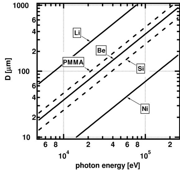
**Figure 4** Material thickness  $D$ , which according to (12) will retard a passing plane wavefield by  $2\pi$  in phase, depending on photon energy for the low-Z elements Li and Be and for pmma, Si and Ni.
