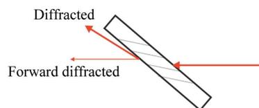
**Figure 2** The Laue-diffracted beam is split into two beams: diffracted and forward-diffracted beams.
