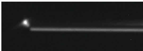
**Figure 1** Image of the beam diffracted from the Laue crystal with the wedge produced in the lateral part of the crystal. The beam diffracted on the wedge is deviated both sagittally and meridionally. A schematic diagram of the diffraction is shown in the lower part of the picture. The width of the wedge was 0.14 mm.
