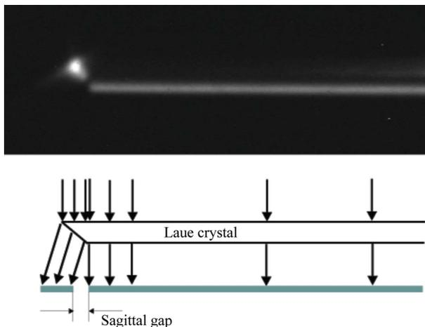
**Figure 1** Image of the beam diffracted from the Laue crystal with the wedge produced in the lateral part of the crystal. The beam diffracted on the wedge is deviated both sagittally and meridionally. A schematic diagram of the diffraction is shown in the lower part of the picture. The width of the wedge was 0.14 mm.
