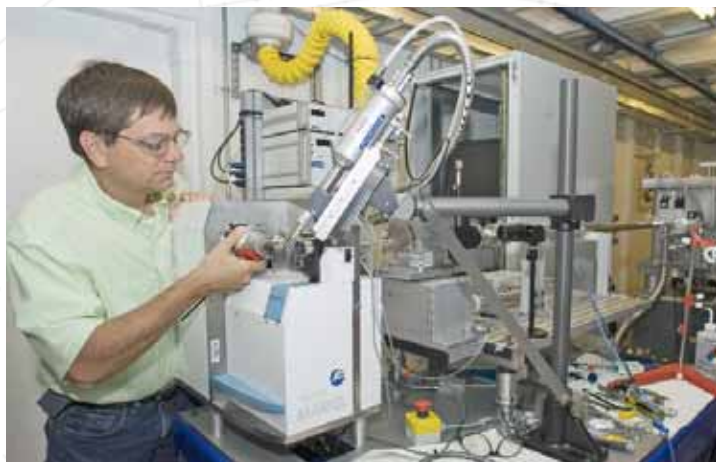
LS-CAT Operations Manager Keith Brister (Northwestern Univ.) at the MD2 diffractometer in the 21-ID-D enclosure.
