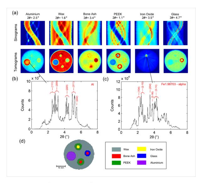
Object reconstruction for angle-dispersive diffraction data. Whilst the reconstructed phases appear accurate, phase identification was almost impossible without prior knowledge of the sample composition. For example it was not possible to conclusively say that the iron oxide phase was hematite, as was identified using EDD data. Therefore, TADDI for large objects holds no apparent advantage over say standard X-ray absorption tomography.
