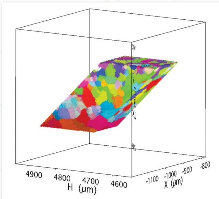
Orientations in a 3-D volume of aluminum. Each color represents a different orientation; the grains show themselves as volumes of constant color. The top is the only external surface, the height of the visible volume is 212  $\mu\text{m}$ , and the base of the volume is 135 x 186  $\mu\text{m}$ . The average rms orientation error for all of the measured points is than 0.01°. Image courtesy of John Budai, Oak Ridge National Laboratory.
