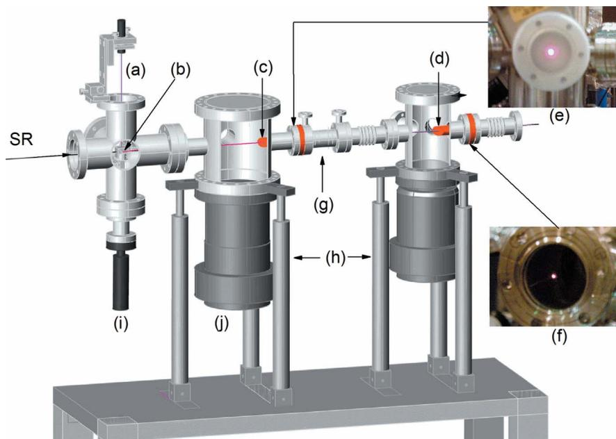
**Figure 2** Installation on site of a two-stage differential pumping system with the compact system for laser alignment: (a) laser beam, (b) beam splitter, (c) first capillary, (d) second capillary, (e) first beam-spot image, (f) second beam-spot image, (g) gas cell, (h) supporting rods, (i) linear feedthrough and (j) turbo pump.
