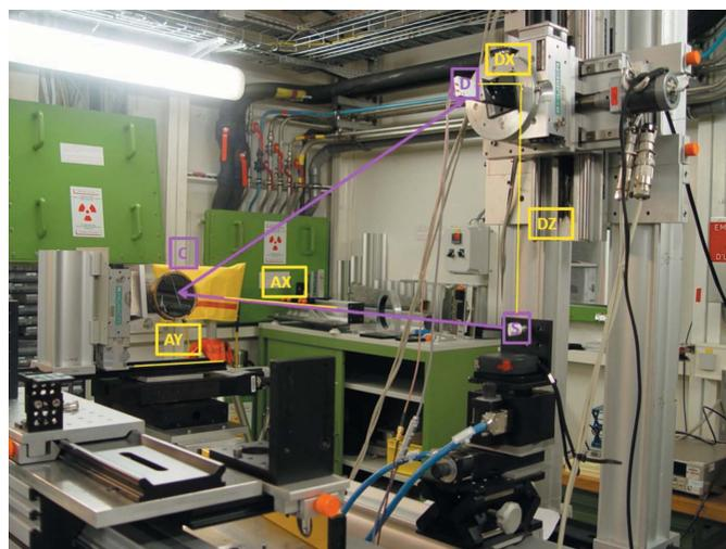
Figure 2 Photograph of the X-ray emission spectrometer setup at the Rossendorf beamline. The positions of the sample (S), crystal (C) and the detector (D) are marked by the respective letters in pink. The linear stages of the crystal analyzer and the detector are shown in yellow and marked as AX, AY and DX, DY
