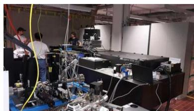
The experimental laser is an important component for performing time resolved optical pump - X-ray probe experiments at SwissFEL. Only a very high reliability and reproducibility guarantees successful experiments. Flexibility in wavelength is achieved by subsequent optical parametric amplification of the laser output. In a synergy between different research groups at PSI, the SwissFEL Experimental Laser 1 is successfully delivered and installed in a temporary Laser lab. Read more:
