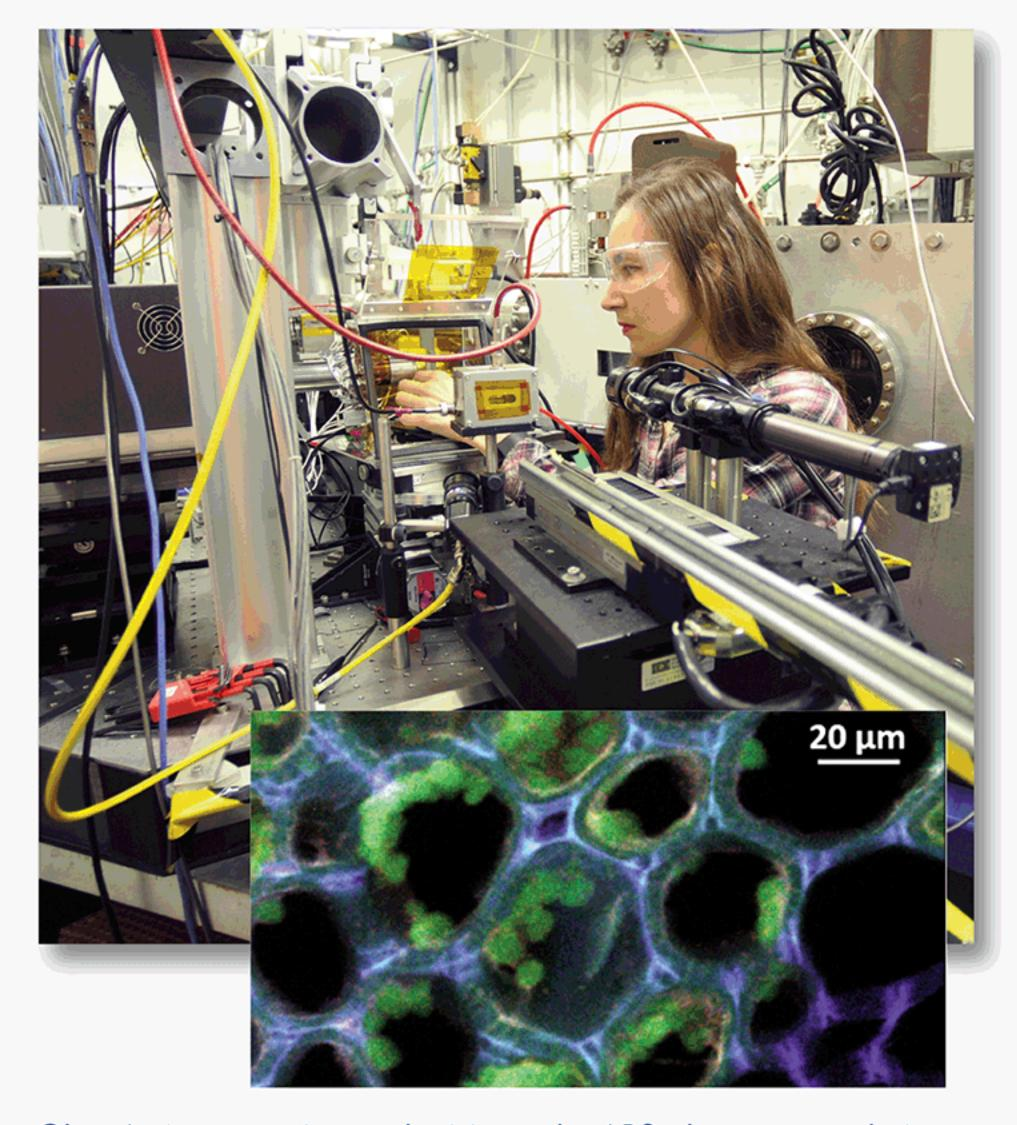
Olga Antipova, assistant physicist at the APS places a sample in xray fluorescent microprobe at the APS 2-ID-E beamline. This instrument is used for imaging and quantification of various elements in biological and other samples, critical for understanding of numerous normal and pathological processes. Inset: Distribution of phosphorus (red), calcium (blue) and elevated levels of potassium (green) within 10-µm thin section of Manchurian ash wood, which is resistant to the emerald ash wood borer.
