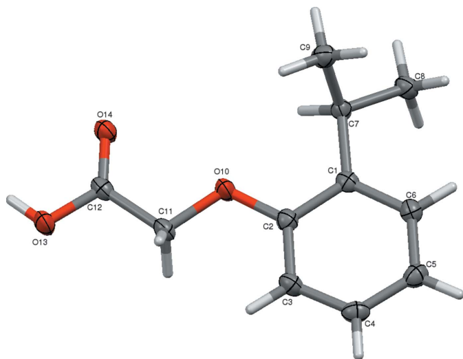
Figure 1 A view of the molecular structure of the title compound, showing the atom labelling. Displacement ellipsoids are drawn at the 50% probability level.
