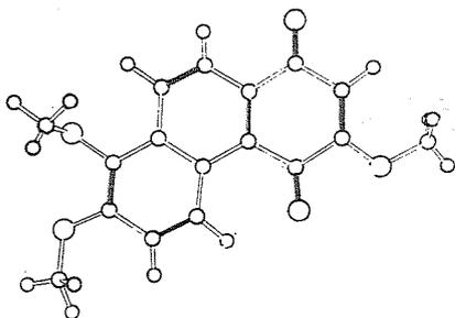
(II):  $P2_1/c$ ,  $D_x = 1.405 \text{ Mg m}^{-3}$ ,  $Z = 4(\text{C}_{17}\text{H}_{14}\text{O}_5)$ ,  $a = 8.442(1)$ ,  $b = 25.129(1)$ ,  $c = 6.717(1) \text{ \AA}$ ,  $\beta = 98.18(1)^\circ$ ,  $1881 \text{ refl.} > 3\sigma(I)$ .
