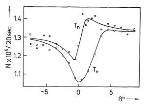
The above displayed figure represents the experimentally measured transmission curves for nonvibrating crystal  $(\mathsf{T}_n)$  and for the same crystal vibrating at a frequency of 2.26 MHz  $(\mathsf{T}_v)$ , excited into vibrations by means of piezoceramic BaTiO $_2$ . The restoration of the AT effect depends on the vibration amplitude and as such may be easy controlled.
