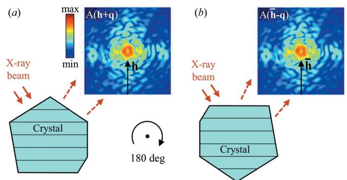
**Figure 1** Schematic diagrams of the multiwavelength anomalous Bragg CDI approach. (a) First, Bragg CDI datasets for the  $\mathbf{h}$  reflection are collected at two photon energies: on the absorption edge of the anomalously scattering atom and several electronvolts below it. (b) Second, the sample is rotated by 180°, and then both measurements are repeated, thus providing two Bragg CDI datasets for the  $\bar{\mathbf{h}}$  reflection.
