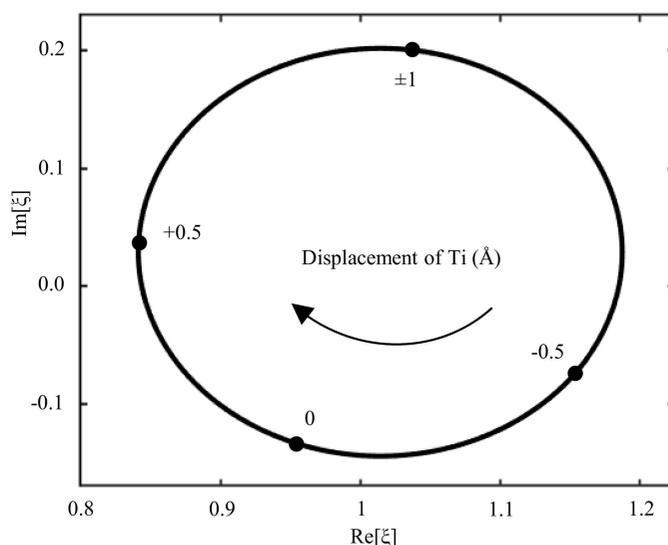
**Figure 4** Parameter  $\xi$  calculated for the (002/00 $\bar{2}$ ) reflections of BaTiO<sub>3</sub>, the Ti  $K$  absorption edge, and the Ti atom displacements in the range of  $[-1; 1]$  Å. Real ( $x$  axis) and imaginary ( $y$  axis) parts of parameter  $\xi$  are plotted. The arrow and labels mark Ti atom displacement along the [001] direction in the tetragonal unit cell of BaTiO<sub>3</sub>.
