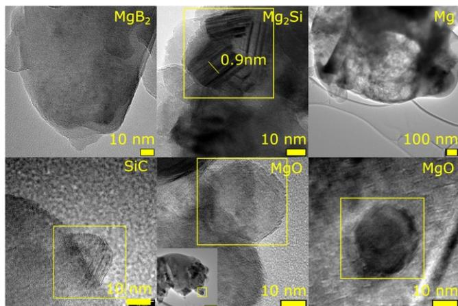
**Figure 1.** TEM images of compounds present in the sintered material.
