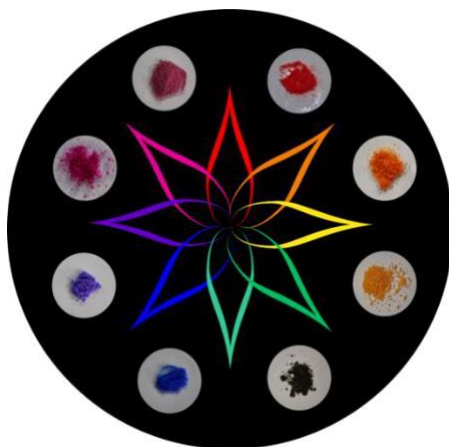
Figure 1. Full-colour palette from one chromogen – multicomponent chromic materials based on violuric acid.
