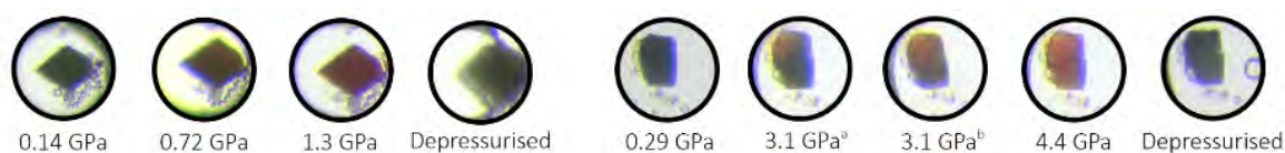
Figure 1. Colour changes in the single-crystal samples of VT active metal-complexes upon application of hydrostatic pressure using a Merrill-Bassett DAC.
