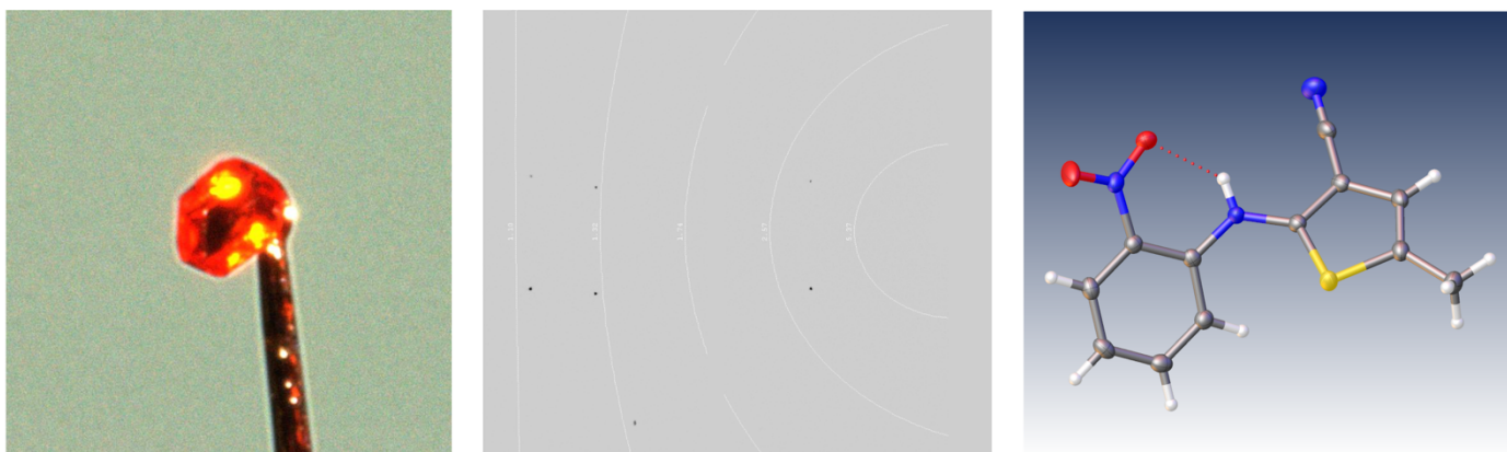
Figure 1. A crystal of 5-methyl-2-((2-nitrophenyl)amino)-3-thiophencarbonitrile (left) and the corresponding crystal structure (right). The steps between the two rely on the diffraction images (centre)
