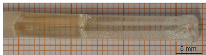
Figure 5 MgO crystal M2/3 grown sequentially with a total length of about 35 mm (about 13 mm for M2 and 22 mm for M3). M2 shows a slightly yellowish tint and the second half of the boule is ‘water clear’. The grid size is one mm by one mm.
