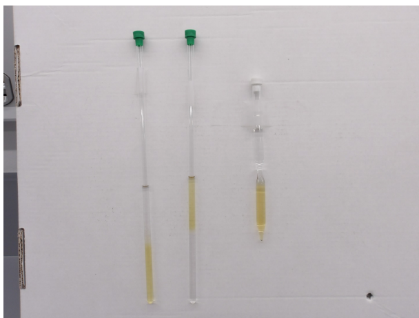
Figure 2 NMR tube prepared for crystallization by (left) layering heptane onto a yellow THF solution, (middle) layering a yellow THF solution onto dichloromethane counter-solvent and (right) layering solution/counter-solvent in a lab-built constriction tube made from a Pasteur pipet.
