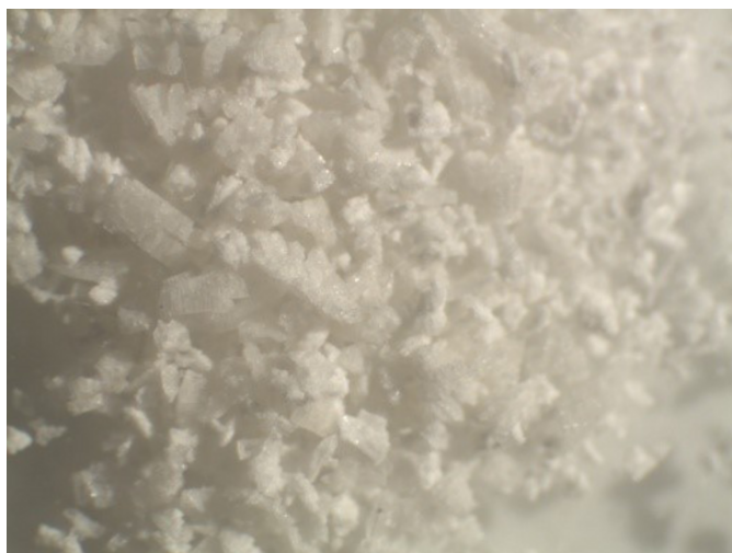
Figure 12 Powder formation generally implies the material came out of solution too fast.
