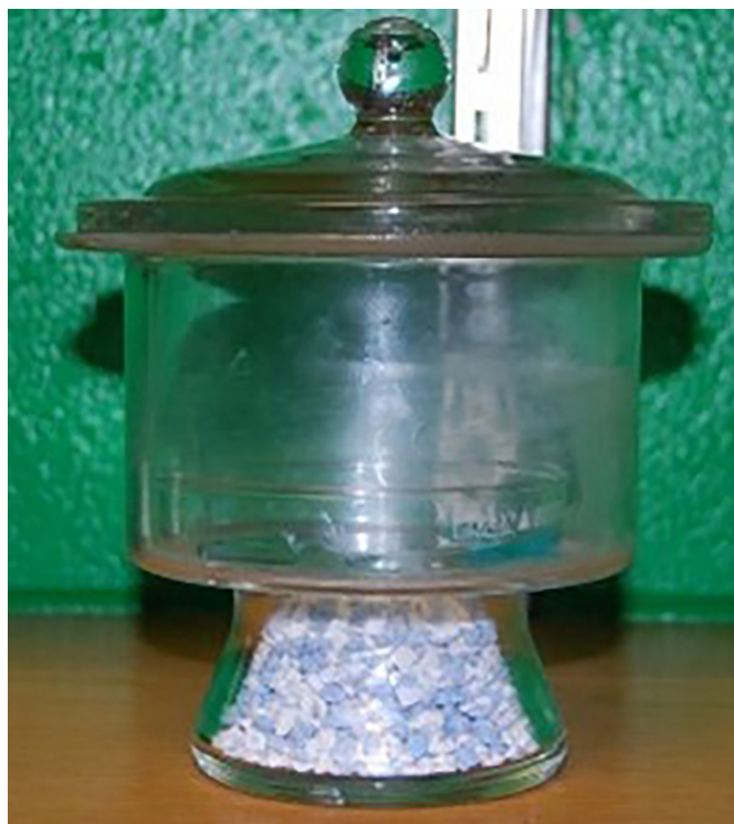
Figure 5 Evaporation inside a desiccator can speed or even control evaporation.
