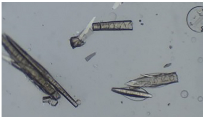
Figure 13 Appearance of cracks in the crystal can mean that there is solvent loss.
