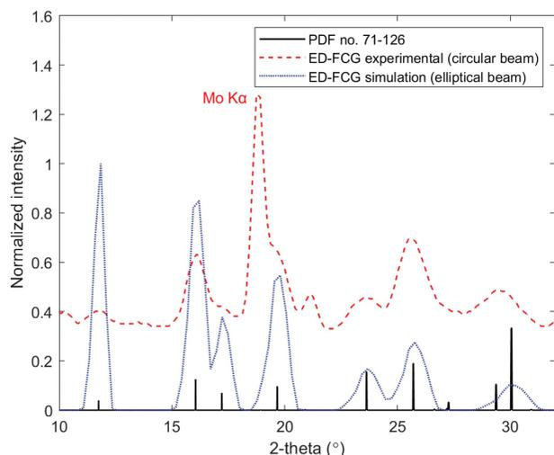
**Figure 8** Energy-dispersive FCG scattering profiles acquired from the NIST corundum plate specimen via a  $\theta:2\theta$  parafofocusing acquisition with a circular collimator (experimental data) and an elliptical collimator (simulated data). The standard peaks of corundum are provided for reference (ICDD PDF card No. 71-126).
