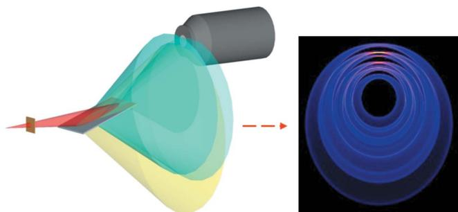
**Figure 1** 3D schematic of a parafofocusing reflection FCG arrangement, illustrating the convergence of four scattering maxima arising from the extreme points along the incident beam's footprint onto the specimen, and a simulated example of the scattering distribution from a 0.5 mm-thick corundum specimen.
