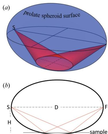
**Figure 2** (a) The surface that satisfies conditions for parafofocusing at a specific scattering angle where the X-ray source, S, detector position, F, and elliptical footprint on a planar specimen are indicated. (b) A cross section through the prolate spheroid for clarity. Note this is not a focusing circle.
