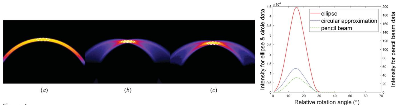
**Figure 4** Simulated reflection FCG images illustrating the convergence of scattering maxima from reflection 111 from an aluminium plate as acquired with (a) a pencil beam, (b) an elliptical collimator and (c) a circular collimator. (d) Intensity changes are quantified in a relative arbitrary scale. Note: data have been integrated around the white dotted lines as the specimen was rotated by a range of angles  $\omega$ .
