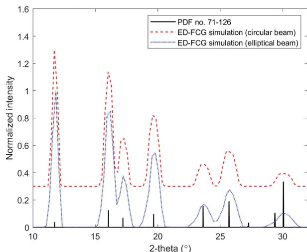
**Figure 7** Simulated energy-dispersive FCG scattering profiles acquired from the NIST corundum plate specimen via a  $\theta:2\theta$  parafofocusing acquisition with a circular collimator and an elliptical collimator. The standard peaks of corundum are provided for reference (ICDD PDF card No. 71-126). Note that the data have been normalized and the circular-beam diffractogram offset for clarity.
