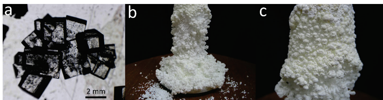
Figure S10. Sodium chloride crystals obtained by slow evaporation crystallization. a) Standard growth of cubic crystals from pure water solution and b) dendritic growth from water solution with addition of \text{K}_4[\text{Fe}(\text{CN})_6]
