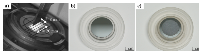
Figure 4 (a) X-ray illuminated area visualized with a fluorescence screen, (b) zero-background plate and (c) zero-background plate with a cavity.
