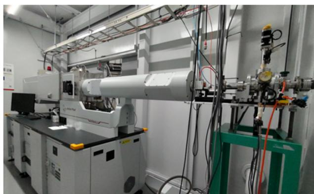
**Figure 1** (Top) Schematic of the BL08W SAXS branch at NanoTerasu. (a) First branch crystal. (b) Second branch crystal. (c) Focusing mirror. (d) Branch crystal for the XRD endstation. (e) Four-quadrant slits. (f) X-ray shutter, absorber and ion chamber. (g) Low-scatter slits. (h) Sample position. (i) Eiger2 1M with a beamstop. (Bottom) Photograph of the apparatus in the hutch.
