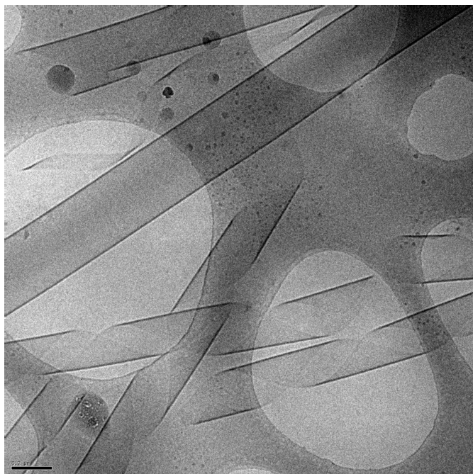
Figure 4 Cryo-TEM image from a 1 wt% solution of C 16 -KKFFVLK.
