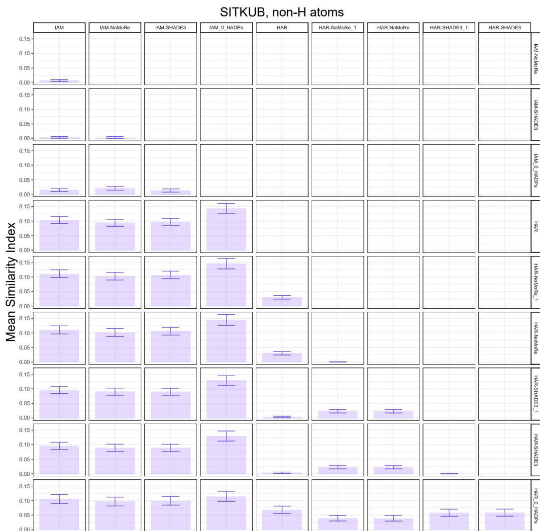
Figure S 39: Mean S_{12} for non-H atoms calculated between the ADPs obtained with various methods. The error bars are estimated standard deviations resulting from error propagation.
