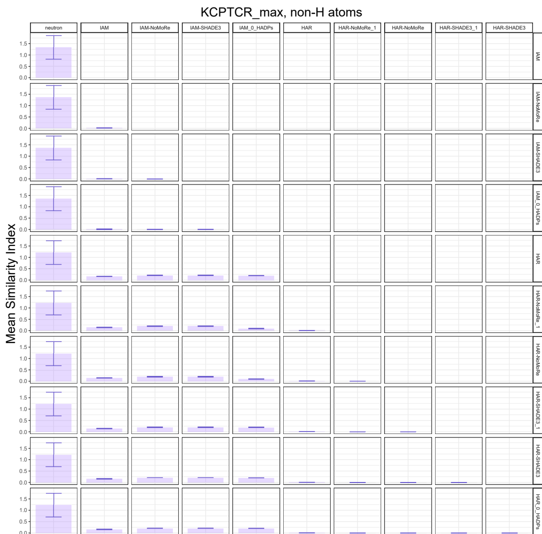
Figure S 43: Mean S_{12} for non-H atoms calculated between the ADPs obtained with various methods. The error bars are estimated standard deviations resulting from error propagation.
