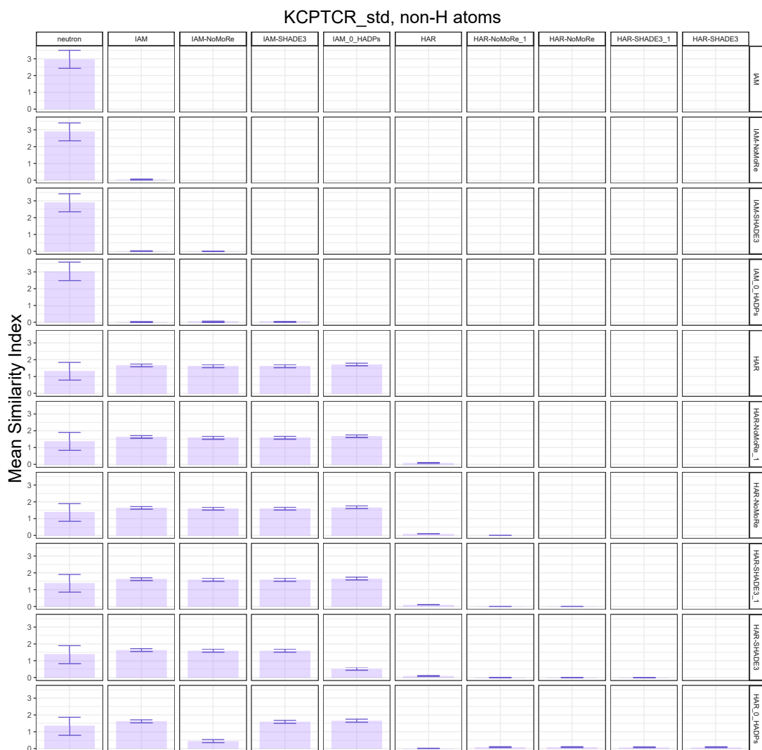
Figure S 44: Mean S_{12} for non-H atoms calculated between the ADPs obtained with various methods. The error bars are estimated standard deviations resulting from error propagation.
