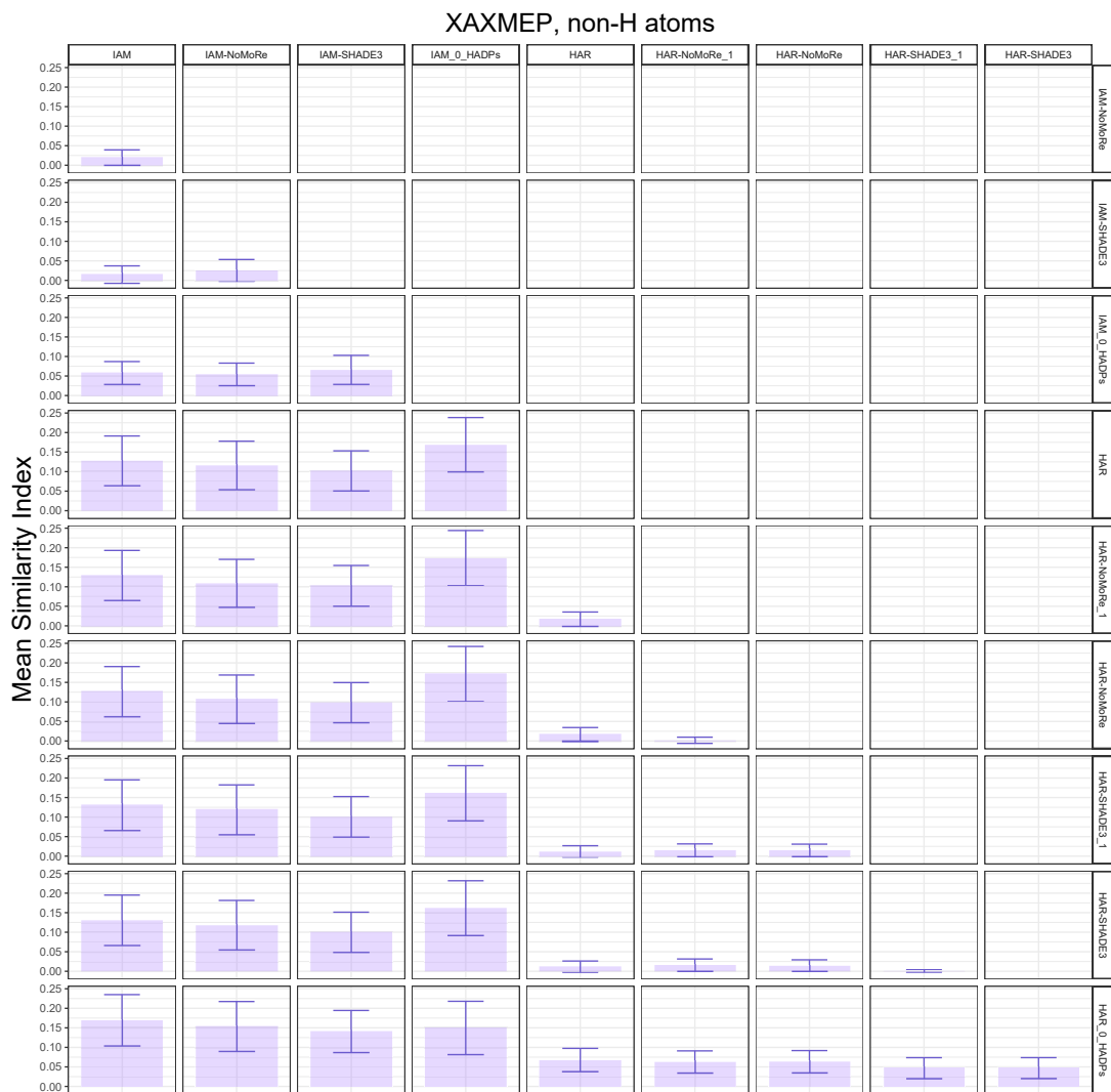
Figure S 41: Mean S_{12} for non-H atoms calculated between the ADPs obtained with various methods. The error bars are estimated standard deviations resulting from error propagation.
