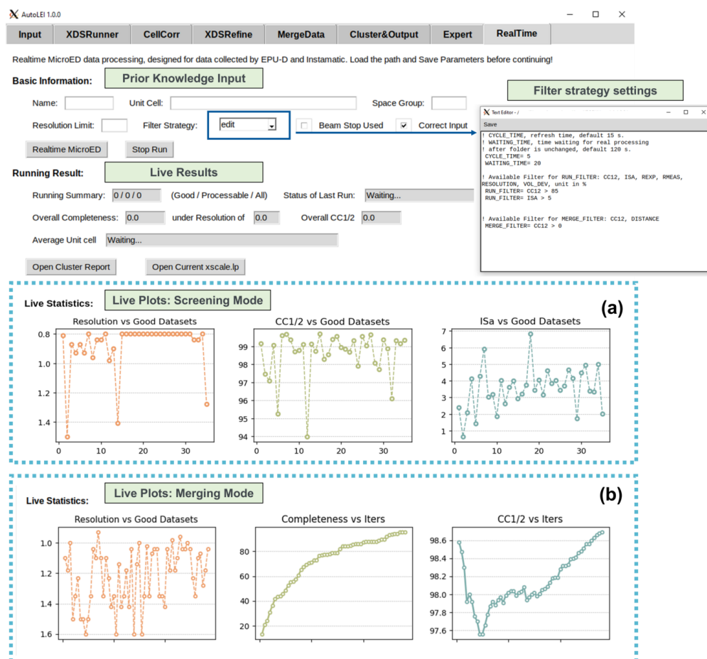
Figure 2 RealTime microED work page. (a) Screening mode. (b) Merging mode. ‘Iters’ in (b) denotes the number of merging iterations.
