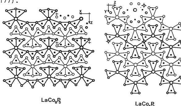
Fig. 1. Comparison of the crystal structures of  $LaCo_8P_5$  and  $LaCo_5P_3$ . The trigonal prisms of metal atoms (large circles:La, small circles:Co) around the P atoms (filled circles) are emphasized. Atoms connected by thin and thick lines are separated from each other by half a translation period of the projection direction.
