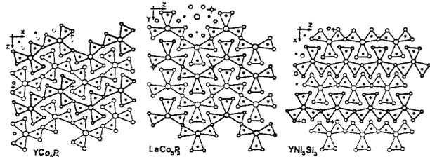
Fig. 2. Similarities of the structures of  $YCo_5P_3$ ,  $LaCo_5P_3$  and  $YNi_5Si_3$  ( $UNi_5Si_3$  type). The trigonal prisms of metal atoms (large and small circles for the rare earth and transition metals respectively) around the metalloid atoms (black dots) are emphasized. Atoms connected by thin and thick lines are separated from each other by half a translation period of the projection direction.
