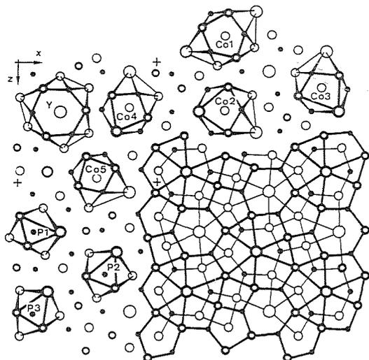
Fig. 1. Crystal structure and near-neighbor coordinations of  $YCo_5P_3$ . Atoms connected by thin and thick lines are at  $y = 1/4$  and  $3/4$  respectively. The coordination polyhedra all have mirror planes perpendicular to the projection direction.
