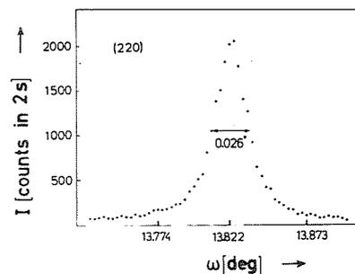
Fig. 2  $\omega$ -scan of the (220) reflection
